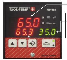
\_Set temperature (required temperature) Adjustable in <sup>1</sup>/10° range
