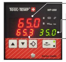
Set temperature (required temperature) Adjustable in <sup>1</sup>/10° range
