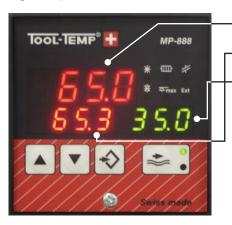
Set temperature (required temperature) Adjustable in <sup>1</sup>/<sub>10</sub>° range
